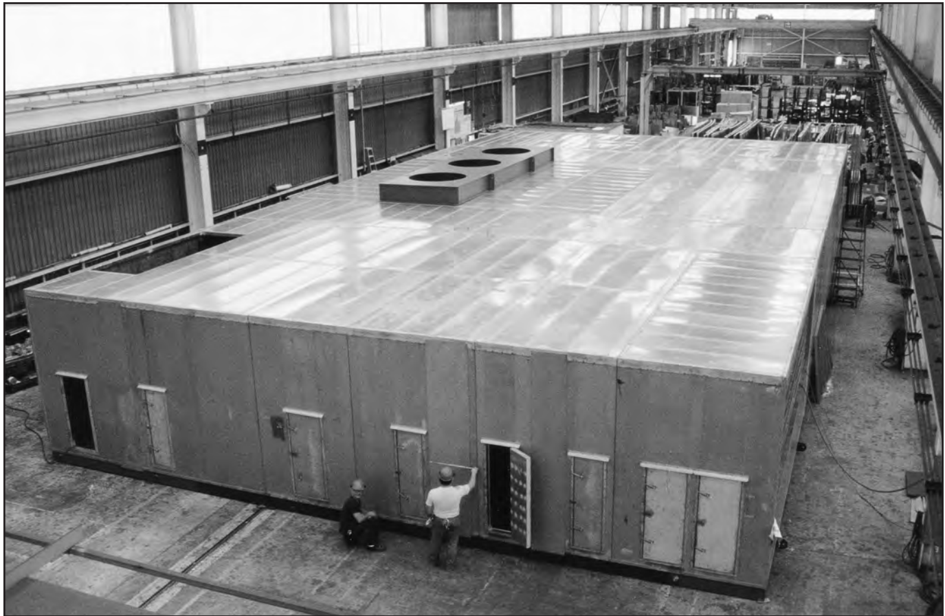
Buffalo Air Handling has the facility and capability to manufacture large air handling units.
