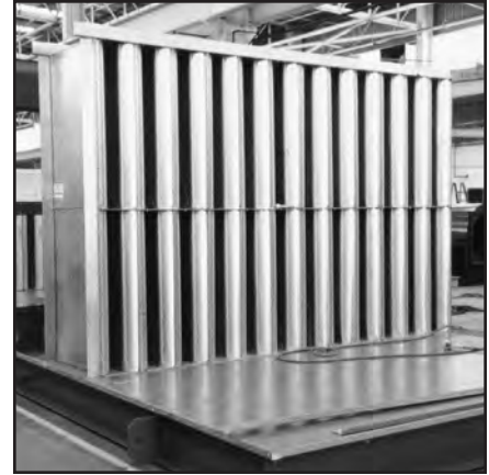
Illustrated is a bank of sound attenuators.
