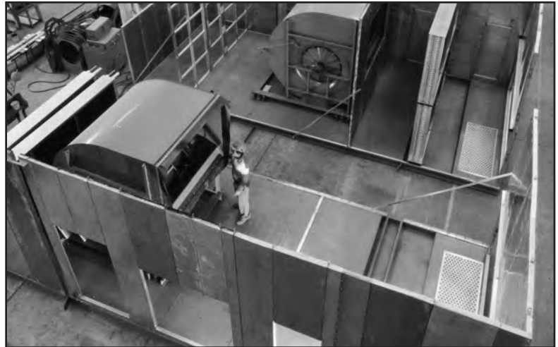
Internal vibration on an all-welded structural steel channel base is essential for reliable fan performance. High pressure and critical applications may require an inertia vibration base where concrete is field installed. A heavy-duty flexible connection between the fan and unit casing is provided for internally isolated fans.
